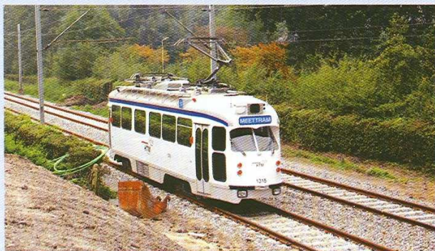
The track monitoring car ('Meettram'), a modified PCC, is the only tram that is allowed on all tracks of the Den Haag network. It is seen in Zoetermeer. K. Pronk
