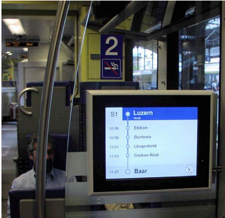
FIGURE 5 – Stadtbahn Zug passenger information video display.
