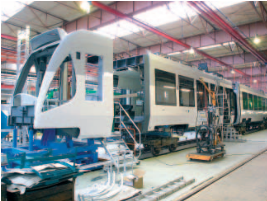
A look into production: Here the new Regio CITADIS for Kassel is built
