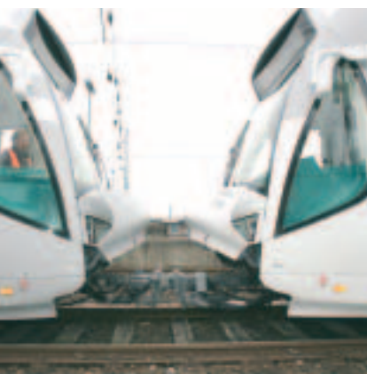
Coupling with electrically elevated nose sections
